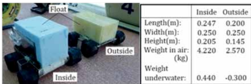
Fig. 8 Improved mobile mechanisms; inside and outside mechanism using magnet tires.
