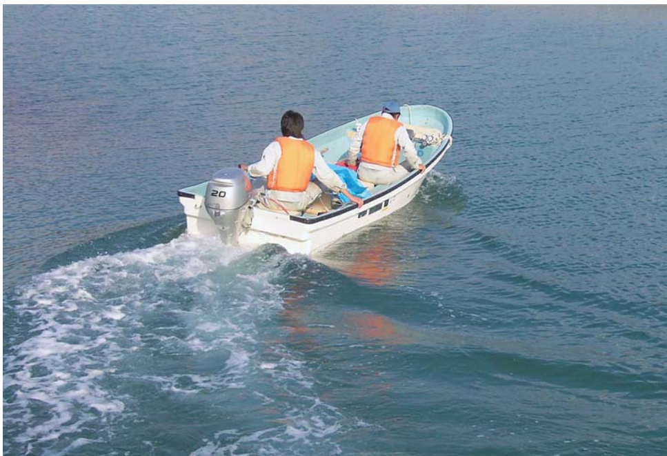
Fig. 2. Test cruising of small boat with hydrogen outboard engine
