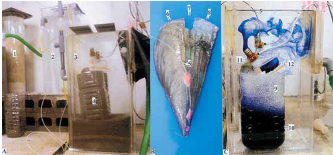
Fig. 1. Experimental system (A and C), operated pen shell (B), and Evans blue discharged from the exhalent orifice (C) in the pen shell. 1 : filter, 2 : water level regulation tank, 3 : respiration chamber, 4 : sand, 5 : polyethylene tubing used for injecting the Evans blue solution to the sand, 6 : inhalent orifice, 7 : notch chipped off the shell for setting the small chamber that catches the water discharged by the pen shell, 8 : exhalent orifice, 9 : acrylic rectangular solid (3 x 2 x 2 mm), 10 : injected Evans blue, 11 : probe of electromagnetic flow-meter, 12 : the small chamber installed at the exhalent orifice.
